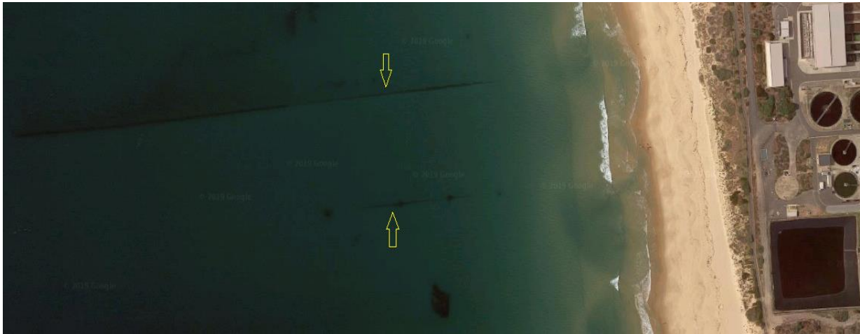
Figure 5. An example of a coastal outfall for Christies Beach WWTP, South Australia.
